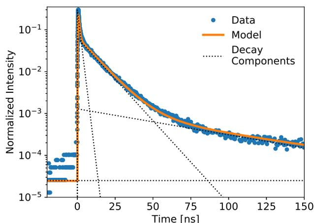
Fig. 5 Showing the components of a 4-exponential fitting (1 rise, 3 decay, plus constant) of the pure LS precursor (90 g/L PPO in LAB) response to a pulsed X-ray source. The data is normalized by integration. Decay lifetimes and weight fractions for the component fitting of all samples are displayed in Tables 1 and 2. Data collected out to +550 ns were used to fit these decay components.
