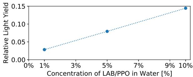
Fig. 7 Relative light yield for the WbLS samples, varying as a function of concentration of LS in water. Each sample was synthesized from a 90 g/L PPO in LAB precursor. Light yield values are presented as a fraction of the EJ-301 light yield. Correction factors have been applied to account for the different X-ray absorption cross-sections between LAB/PPO and water.
