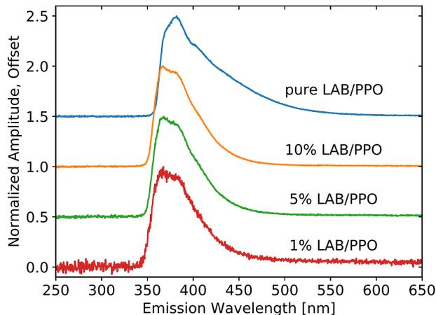
Fig. 2 Emission spectra resulting from X-ray excitation of pure LS (LAB with 90 g/L PPO) and the three WbLS concentrations made from this LS. Each curve is displayed normalized at its maximum and offset along the vertical axis.
