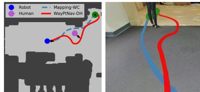
Fig. 3. Top view of the trajectories taken by Mapping-WC and LB-WayPtNav-DH from the same state and the corresponding RGB image with the trajectories superimposed. Mapping-WC reaches the goal faster than LB-WayPtNav-DH as it has access to precise geometry of the scene and the human state and thus plans a path between the human and the wall which narrowly avoids collision. LB-WayPtNav-DH, on the other hand, takes a more cautious path as it does not have access to the human state.
