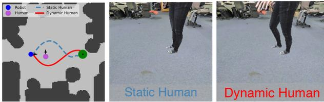
Fig. 4. Top view of the trajectories taken by LB-WayPtNav-DH from the same state with a static human (light blue, dashed line) and a dynamic human (red, solid line), and the corresponding RGB images. HumANav enables LB-WayPtNav-DH to leverage cues, such as spread of humans legs and direction of human toes, to infer that the left RGB image likely corresponds to a static human and the right one to a moving human.
