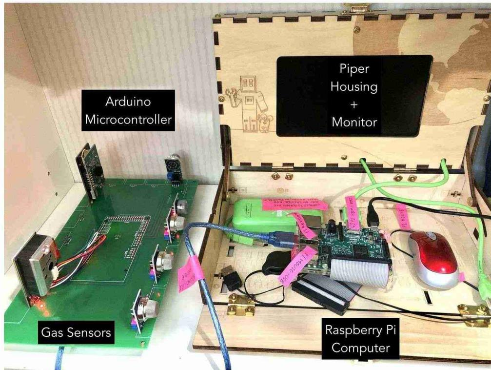
Figure 5.8: **Custom Gas Sensor IoT Device.** This sensor IoT system was built with multiple gas sensors connected to an Arduino micro-controller that links to a Raspberry Pi computer. The computer sends the signal via a web Rest-API that allows for a minute by minute monitoring of the gases in the local environment.
