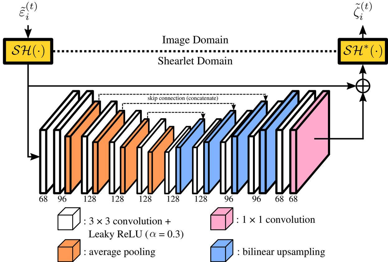
Figure 2. Architecture of the deep convolutional network of CycleST, referred to as  $\mathcal{R}(\cdot)$ . Based on the U-Net architecture [25] and residual learning strategy [26],  $\mathcal{R}(\cdot)$  refines the shearlet coefficients of  $\tilde{\varepsilon}_i^{(t)}$  in shearlet domain to produce inpainted  $\tilde{\zeta}_i^{(t)}$  in image domain.
