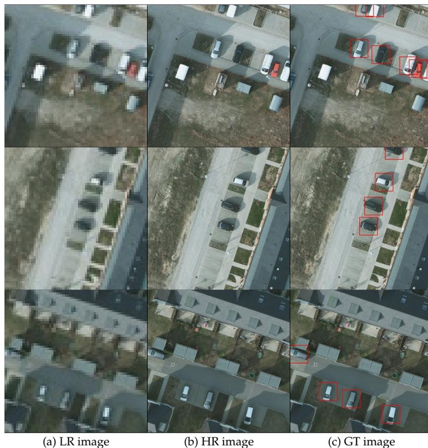
**Figure 6.** COWC (car overhead with context) dataset: LR-HR (low-resolution and high-resolution) image pairs are shown in (a) and (b) and GT (ground truth) images with bounding boxes for cars are in (c).
