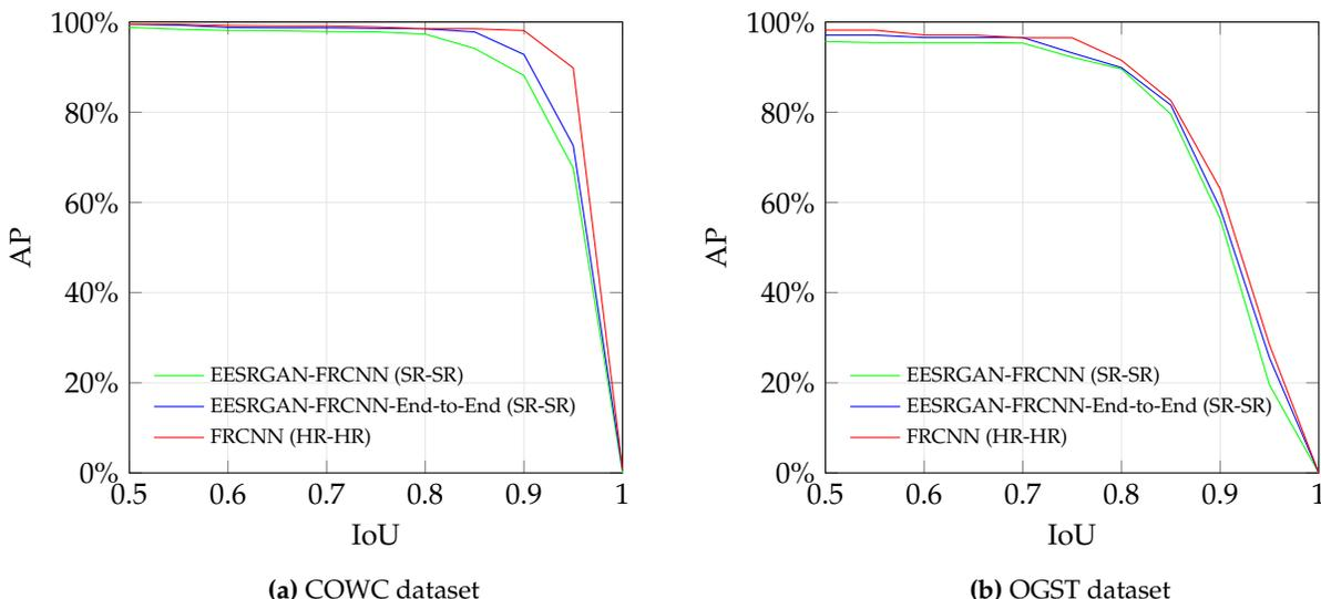
**Figure 8.** AP-IoU (average precision-intersection over union) curves for the datasets. Plotted results show the detection performance of standalone faster R-CNN on HR (high-resolution) images and our proposed method (with and without end-to-end training) on SR (super-resolution) images.
