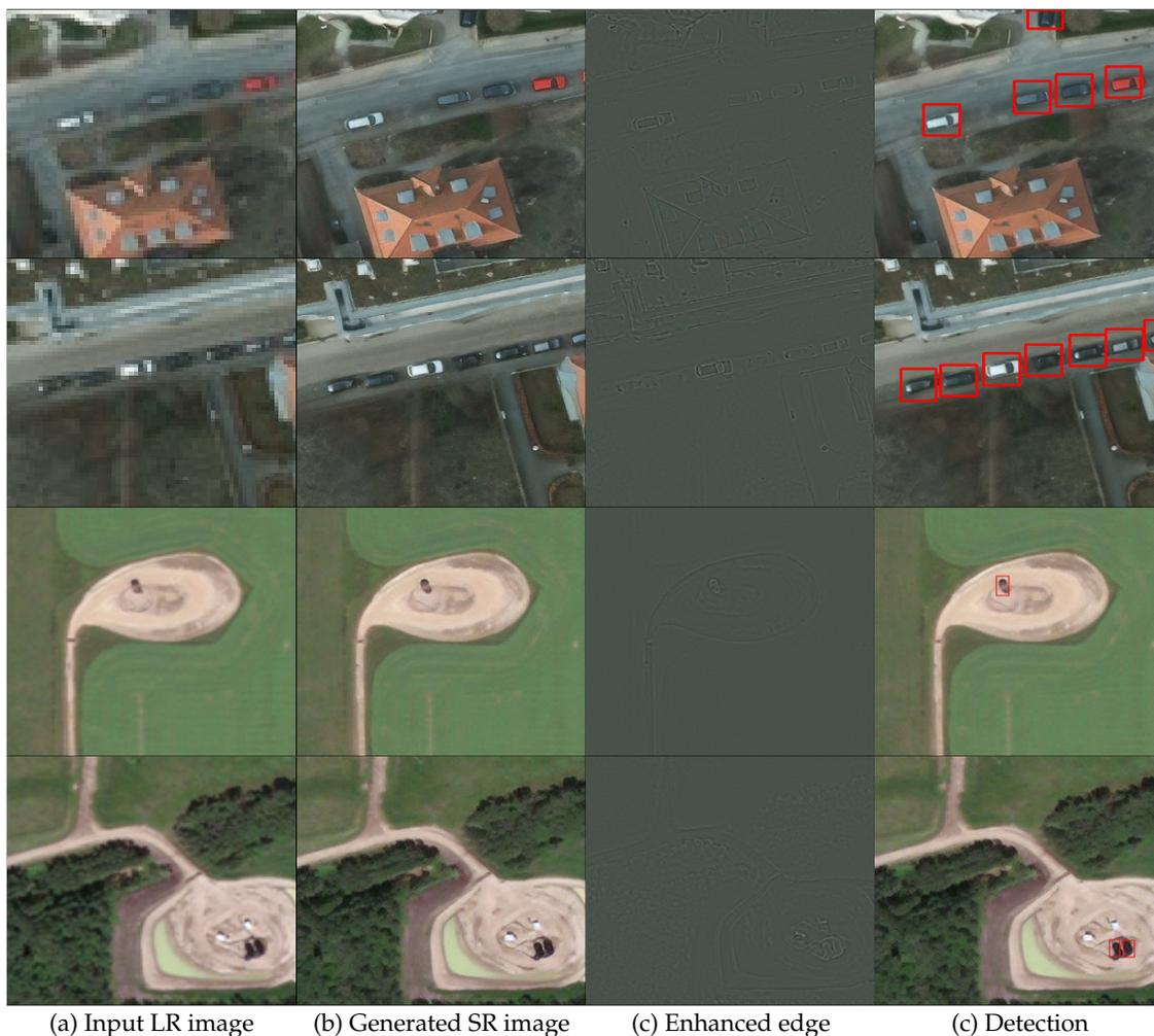
**Figure 11.** Examples of SR (super-resolution) images that are generated from input LR (low-resolution) images are shown in (a) and (b). The enhanced edges and detection results are shown in (c) and (d).
