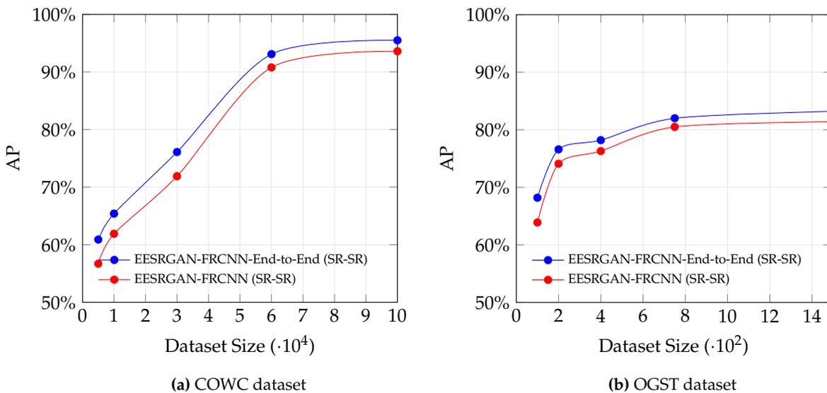
**Figure 10.** AP (average precision) with varying number of training sets from the datasets. Plotted results show the detection performance of our proposed method (with and without end-to-end training) on SR (super-resolution) images.
