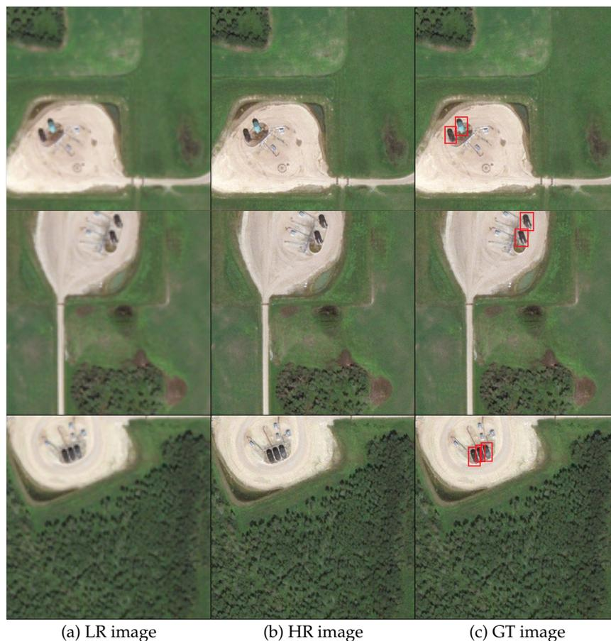
**Figure 7.** OGST (oil and gas storage tank) dataset: LR-HR (low-resolution and high-resolution) image pairs are shown in (a) and (b) and GT (ground truth) images with bounding boxes for oil and gas storage tanks are in (c).
