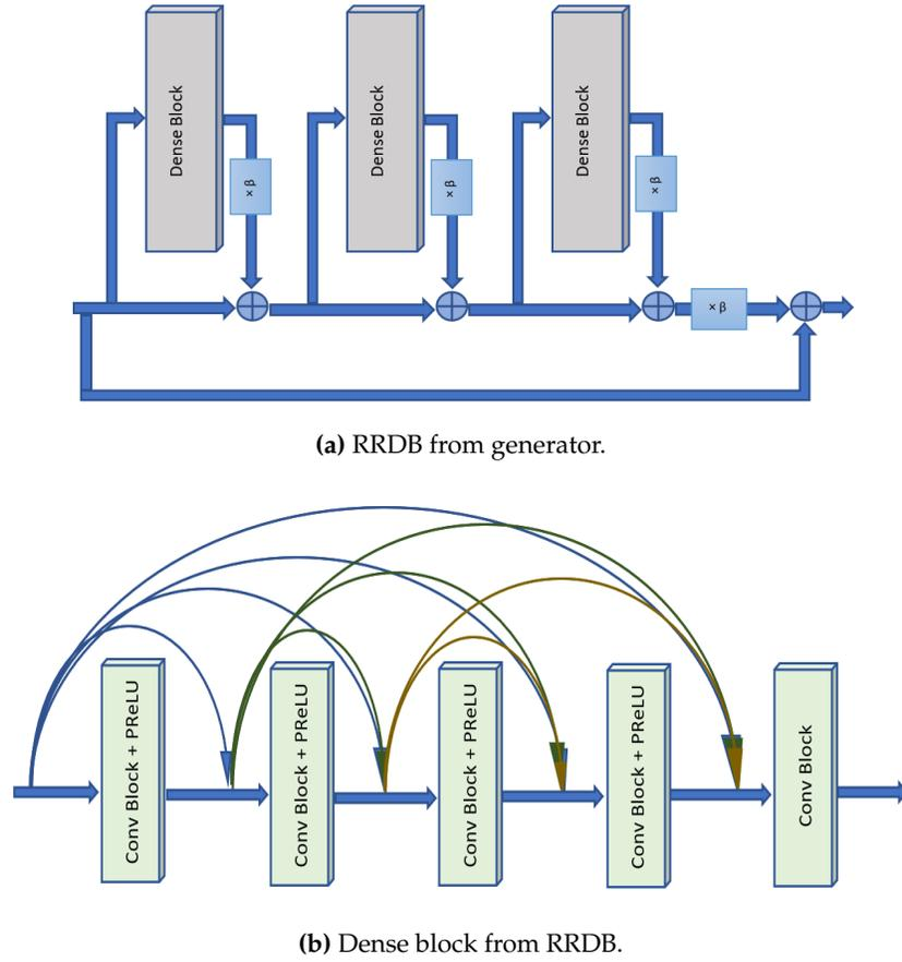
**Figure 4.** Internal diagram of RRDB (residual-in-residual dense blocks).
