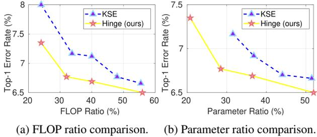
Figure 4: (a) FLOP and (b) parameter comparison between KSE [28] and Hinge under different compression ratio. ResNet56 is compressed. Top-1 error rate is reported.
