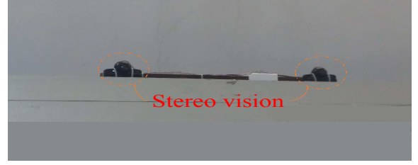
(b) The prototype of a stereo vision system, which is attached to the ceiling of laboratory in the geometrical center of the top of the workspace.
