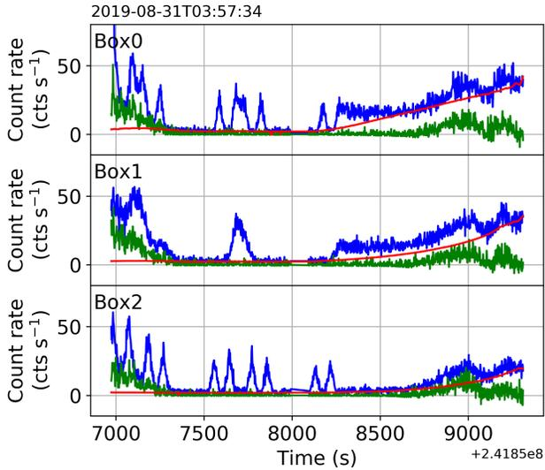
**Figure 6.** LE light curves with the normal scanning and data download mode. The blue and green curves are light curves of 1 – 6 keV and 8.6 – 10.3 keV, respectively. The red curves are the backgrounds calculated by the SNIP method.
