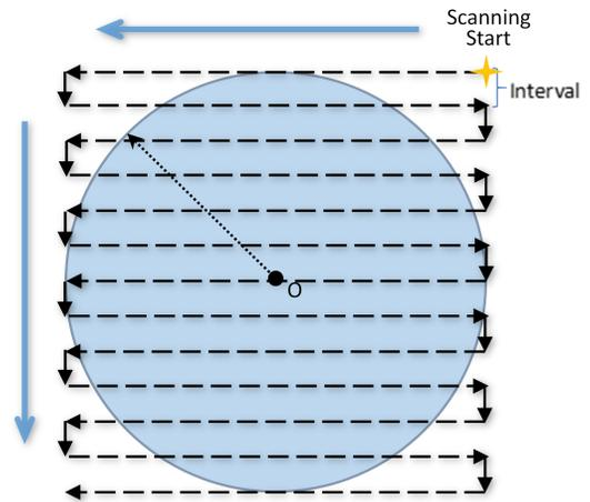
**Figure 2.** Schematic diagram of a small area scan. “O” is the center of the scanned area and the circle is the observed area. The dotted line with the arrow is the scanning track.
