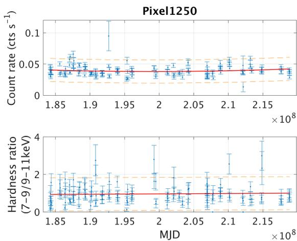
**Figure 8.** Long-term light curve and hardness curve of a typical pixel (blank sky). This figure also shows the fitting functions of count rate and hardness ratio (blue point: blank sky data, red solid line: ideal count rate curve, orange dashed line: ideal count rate limit)
