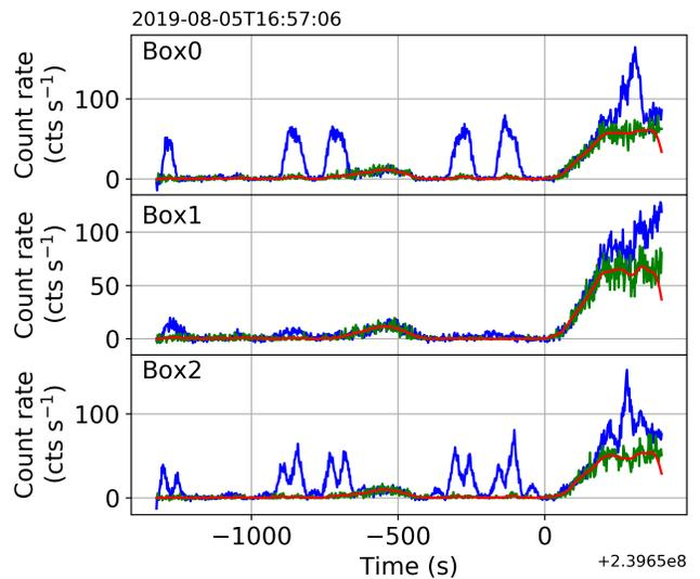
**Figure 5.** LE light curves affected by particle events. The blue and green lines are the light curves in 1 – 6 keV and 8.6 – 10.3 keV, respectively. The red lines are the smoothed green lines. The green bumps on the right end are caused by particle events and need to be removed.
