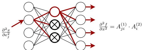
**Fig. 1.** A schematic of our extraction attack on a 1-deep neural network. Let  $x$  be an input that causes exactly one neuron to have value zero. The second differential becomes zero at all other neurons—because they remain either fully-inactive or fully-active. Therefore the value of this differential is equal to the product of the weight going into the neuron at its critical point and the weight going out of this neuron.
