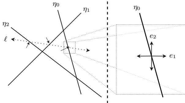
**Fig. 2.** (left) Geometry of a 1-deep neural network. The three solid lines corresponds to “critical hyperplanes” of neurons. We identify one *witness* to each neuron with binary search on the dotted line  $\ell$ . (right) For each discovered critical point, we compute the second partial derivative along axis  $e_1$  and  $e_2$  to compute the angle of the hyperplane.
