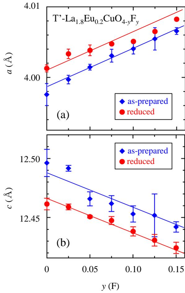
Fig. 2. (color online) Fluorine content  $y$  dependence of the lattice constants (a)  $a$  and (b)  $c$  for as-prepared (diamonds) and reduced (circles) samples of  $T'\text{-La}_{1.8}\text{Eu}_{0.2}\text{CuO}_{4-y}\text{F}_y$ . Solid lines are guides to the eyes.
