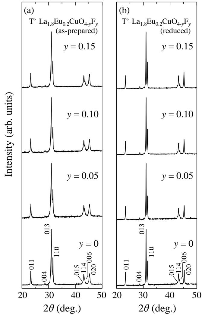
Fig. 1. Powder x-ray diffraction patterns of (a) as-prepared and (b) reduced samples of  $T'-La_{1.8}Eu_{0.2}CuO_{4-y}F_y$  ( $y = 0 - 0.15$ ).
