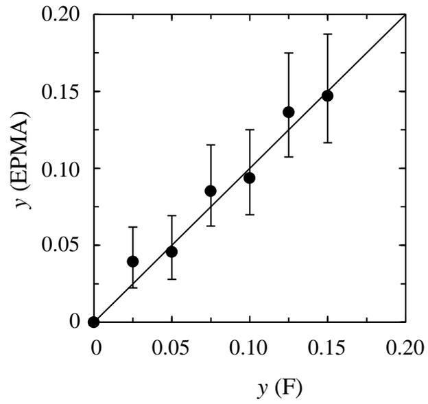
Fig. 3. Dependence of the fluorine content  $y(\text{EPMA})$  estimated by EPMA on the nominal fluorine content  $y$  in reduced samples of  $\text{T}'\text{-La}_{1.8}\text{Eu}_{0.2}\text{CuO}_{4-y}\text{F}_y$ .
