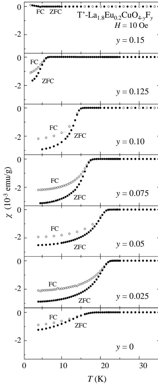
Fig. 4. Temperature dependences of the magnetic susceptibility,  $\chi$ , for reduced samples of  $T'$ - $\text{La}_{1.8}\text{Eu}_{0.2}\text{CuO}_{4-y}\text{F}_y$  measured in a magnetic field of 10 Oe on zero-field cooling (ZFC) (closed circles) and field cooling (FC) (open circles).
