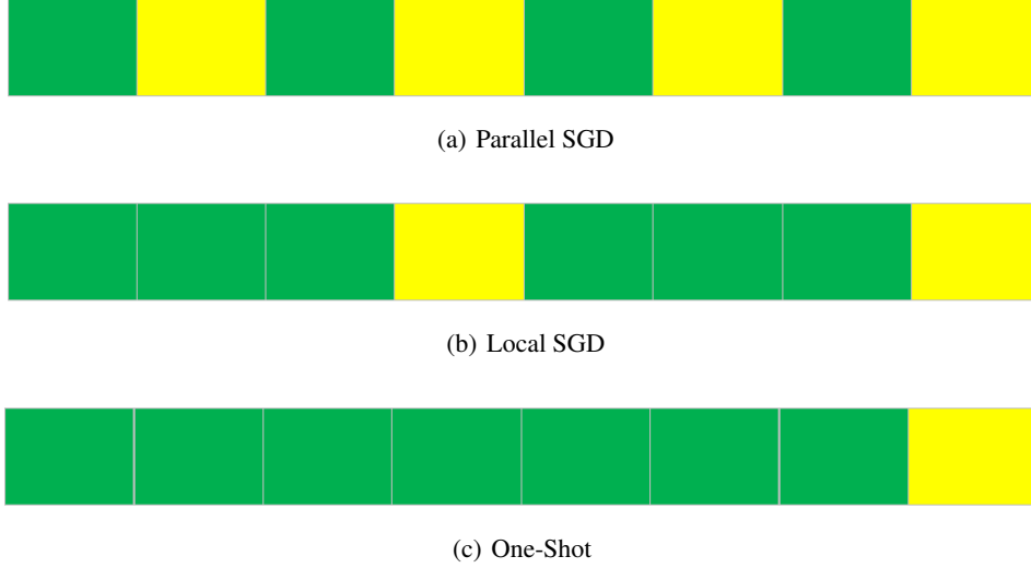
Figure 6: Comparison of vanilla parallel SGD, local SGD and one-shot learning, where a green block indicates computation and a yellow block corresponds to communication.
