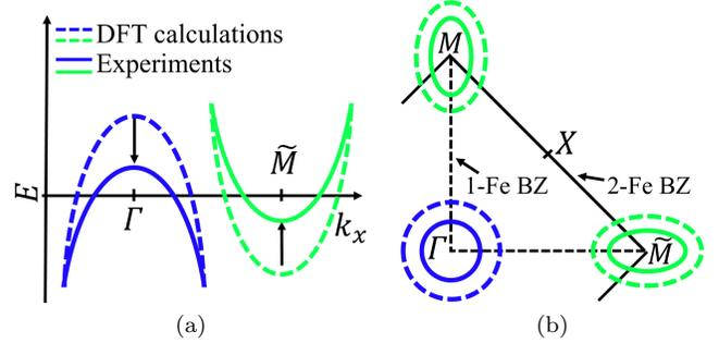
FIG. 1. Schematic plot showing (a) band structure along  $k_x$  direction and (b) corresponding Fermi surface of a generic FeSC in the 1-Fe BZ. The dashed lines represent DFT-predicted  $\Gamma$ -centered hole (blue) and  $\tilde{M}$ -centered electron (green) bands. The solid lines represent the renormalized bands, as observed in dHvA and ARPES experiments, with momentum-dependent energy shifts and shrunken pocket sizes.
