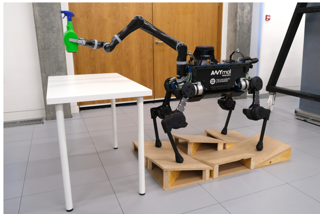
Fig. 1: A legged loco-manipulation system: ANYmal [2] is a fully torque-controlled quadruped robot. We equipped it with a Kinova Jaco [3] robot arm. An accompanying video is available at https://youtu.be/vDesP7IpThw .
