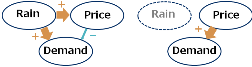
Figure 1: Example with three variables in price optimization. The variables consist of a decision variable "price," a target variable "demand," and an external feature "rain." The portion on the left shows the true causal model, where price has a negative effect on demand, and rain has a positive effect on both price and demand. The portion on the right shows an accurate prediction model, in which high price is related to high demand, a so called "spurious correlation." The rain variable is invisible to the predictor and optimizer and, thus, behaves as an unobserved cofounder.
