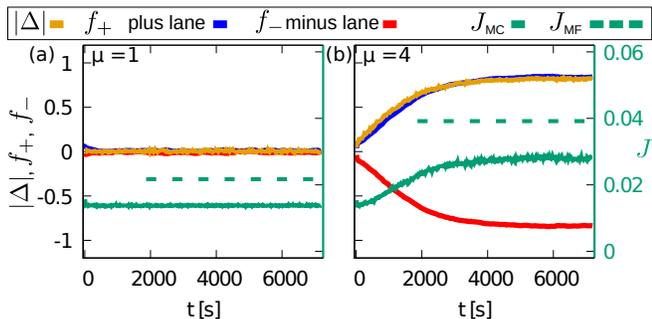
FIG. 2. Time dependence of the flux and particle densities for a system of  $L = 1000$ ,  $\rho = 0.05$ , and random initial configurations. Values of the floor-fields  $f_+$ ,  $f_-$  and difference in densities  $\Delta$  are given at the left axis; values of the total flux  $J$ , and the mean-field estimation  $J_{MF}$  are given at the right axis. (a)  $\mu = 1$ , (b)  $\mu = 4$ .
