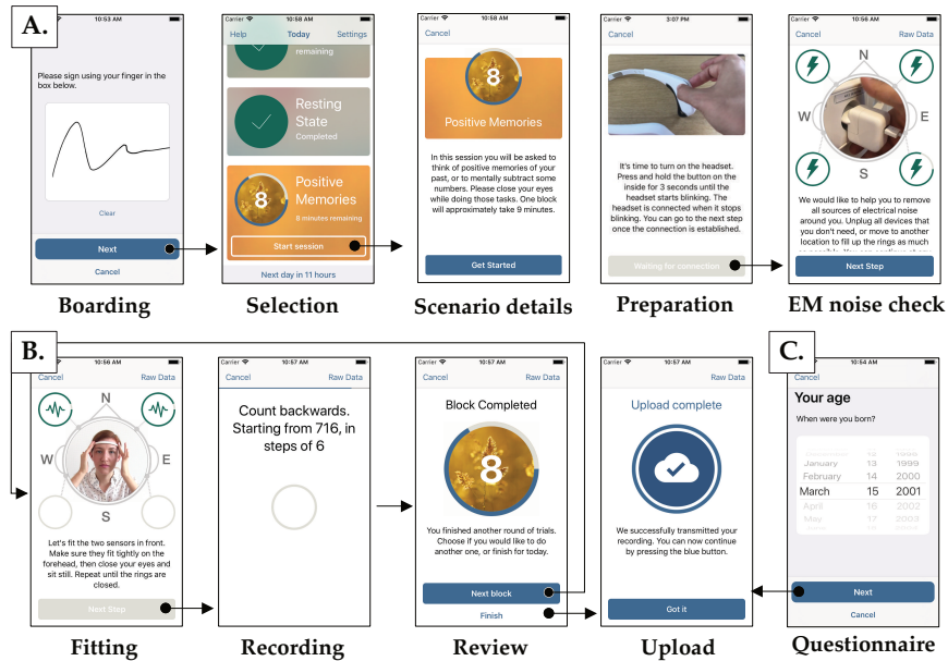
Fig. 1. The user-interface flow of participating in a study with MYND . (A) After boarding and consent review, subjects can select a scenario, inform themselves about the scenario’s tasks, prepare the hardware, and fit a suitable location with the electromagnetic (EM) noise check. (B) A scenario is broken up into several blocks of trials. After each block, subjects can review their progress and choose to proceed to the next block with an intermediate assessment of the hardware’s fit, or end the recording session and upload the recorded data. (C) An exemplary screen of a questionnaire scenario. Multiple-choice, short text answers, and date selection are supported.
