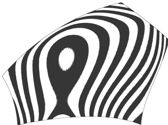
Figure 4: Isophotes of the surface shown in Figure 3c.
