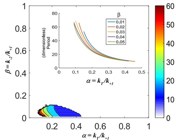
**Figure 6.** Approximate region of stable limit cycle oscillations for design II from numerical integration; colormap shows dimensionless period as the ratio of rates are varied (fixed  $\tilde{Y}_0 = 0.5$ ) and the inset shows the approximate power-law dependence of the dimensionless period on  $\alpha$ .
