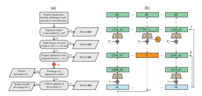
Figure 1: In (a) the block scheme of  $\mathcal{M}^{\mathcal{A}}$  is depicted. A bullet marks a point for UD challenge. In (b) an introducing image and second pre-image challenges in the public key of the W-OTS<sup>+</sup> scheme is shown.
