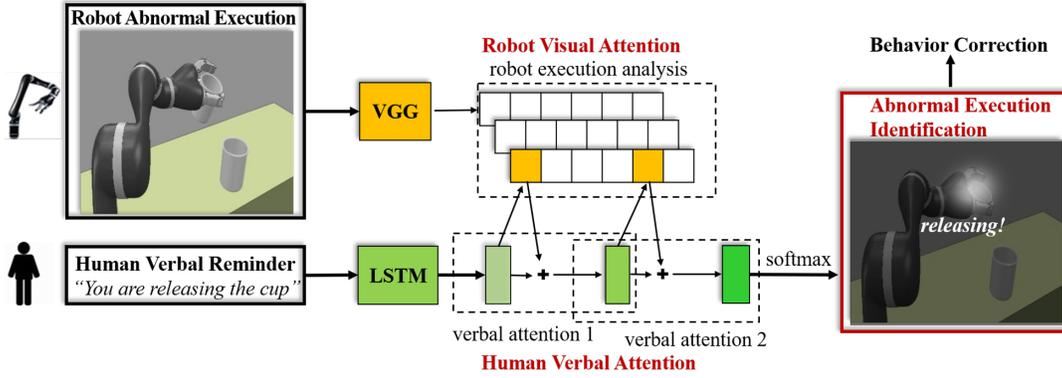
Fig. 2: The framework of *H2R-AT* using human verbal reminders for robot failure avoidance. Human attention is embedded in verbal reminders. Feature vectors extracted from human verbal reminders and feature vectors from robot visual perceiving are combined to get confined attention. With the confined attention, the robot can correct its abnormal behavior accordingly.
