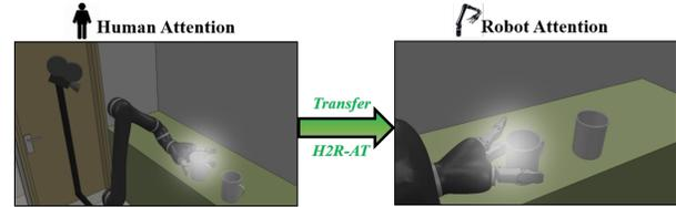
Fig. 1: An illustration of the attention transfer using the developed *H2R-AT* model. The attention region of a human (from human observation perspective) and robot (from robot perceiving perspective) are highlighted as shown. By using *H2R-AT* the attention of abnormal robot executions was transferred from a human to a robot to alert its failures in an early stage before failures happen.
