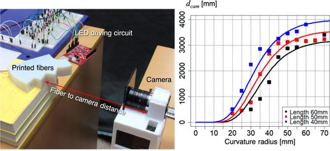
Fig. 7. Measurement of  $d_{cam}$  (the longest distance between a fiber and camera where blinking binary pattern is detectable): (left) measurement setup, (right) result.
