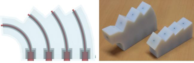
Fig. 6. Printed optical fibers for parameter identification: (left) internal structure, (right) printed fibers.
