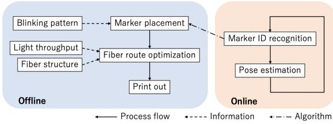
Fig. 2. The overall system diagram.
