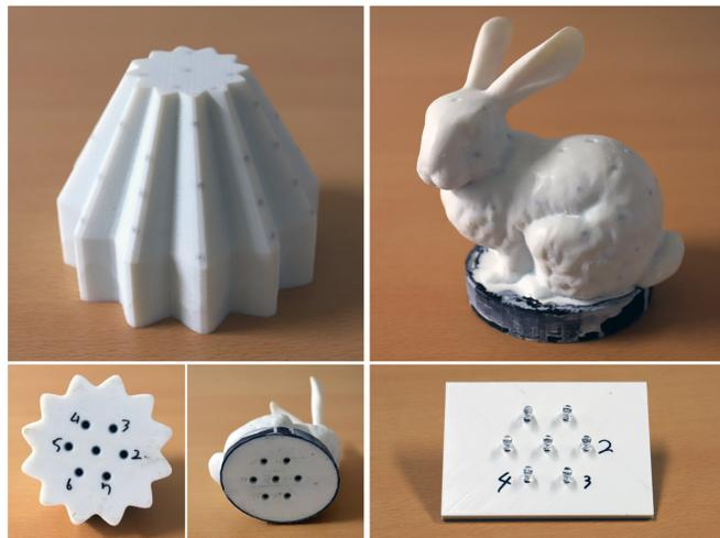
Fig. 9. Printed objects and IR LEDs of the base component (bottom right).
