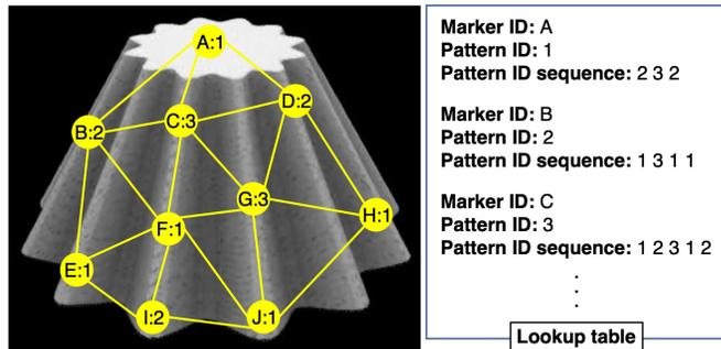
Fig. 3. Example of connected adjacent markers overlaid on a simulated image and a lookup table of the markers.
