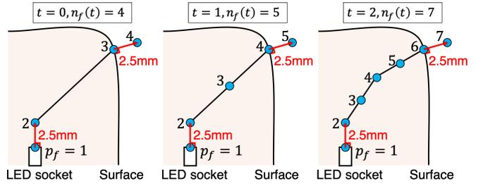
Fig. 8. Initial routing of a printed optical fiber.
