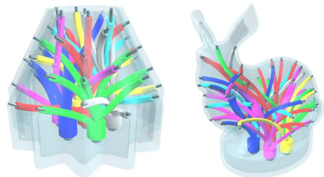
Fig. 10. The internal structures of the printed objects. Fibers with the same color are connected to the same LED.
