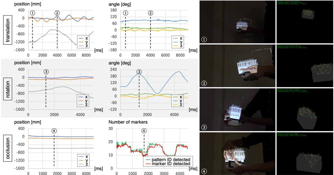
Fig. 14. Projection result of the building object in translation, rotation, and occlusion: (left) the time series of 3D position and orientation of the object in the IR camera coordinate system, and the number of markers whose pattern/marker IDs were detected, (right) captured image of the projected object by the camcorder and visualization of detected markers and estimated pose of the object superimposed in captured image by the camera at frames indicated by the numbers in a circle.
