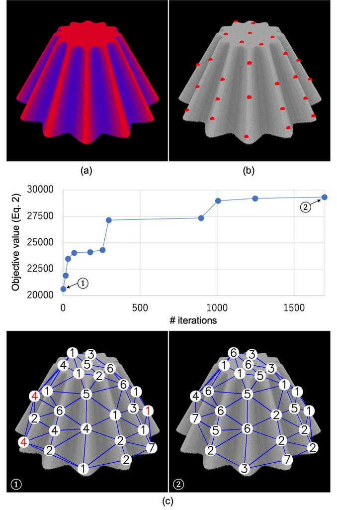
Fig. 4. Marker placement for a wavy cone surface: (a) Visualization of  $s(p_m)$  (red: large, blue: small). (b) Initial candidate marker places as red points. (c) Pattern ID assignment by GA (top: the objective value of Equation 2 is improved in the iterations, bottom: marker assignments at the first and last iterations where red numbers indicate that the marker IDs of these markers cannot be recognized in the simulation).
