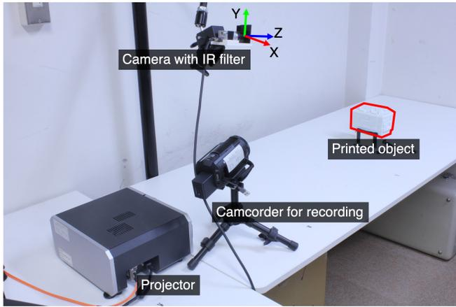
Fig. 11. Projector-camera system. The colored axes show the IR camera coordinate system.
