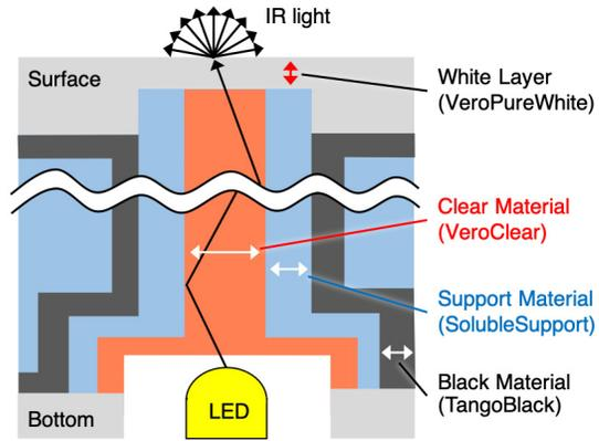
Fig. 5. Optical fiber design.
