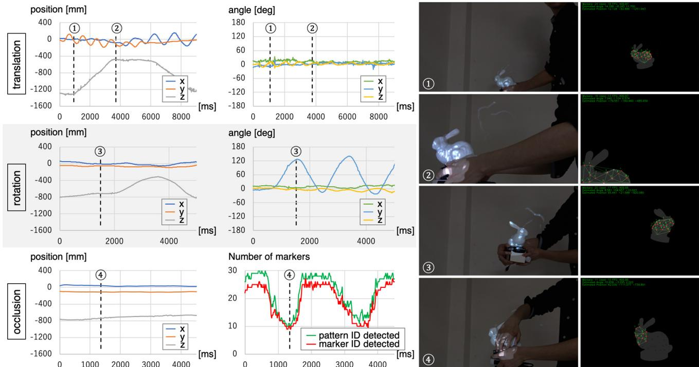
Fig. 13. Projection result of the bunny object in translation, rotation, and occlusion: (left) the time series of 3D position and orientation of the object in the IR camera coordinate system, and the number of markers whose pattern/marker IDs were detected, (right) captured image of the projected object by the camcorder and visualization of detected markers and estimated pose of the object superimposed in captured image by the camera at frames indicated by the numbers in a circle.
