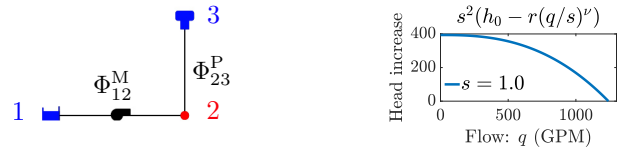
Fig. 6: Three-node network(left) and its variable-speed pump curve (right). The \Phi(\cdot) function denotes nonlinear head loss or head gain.
