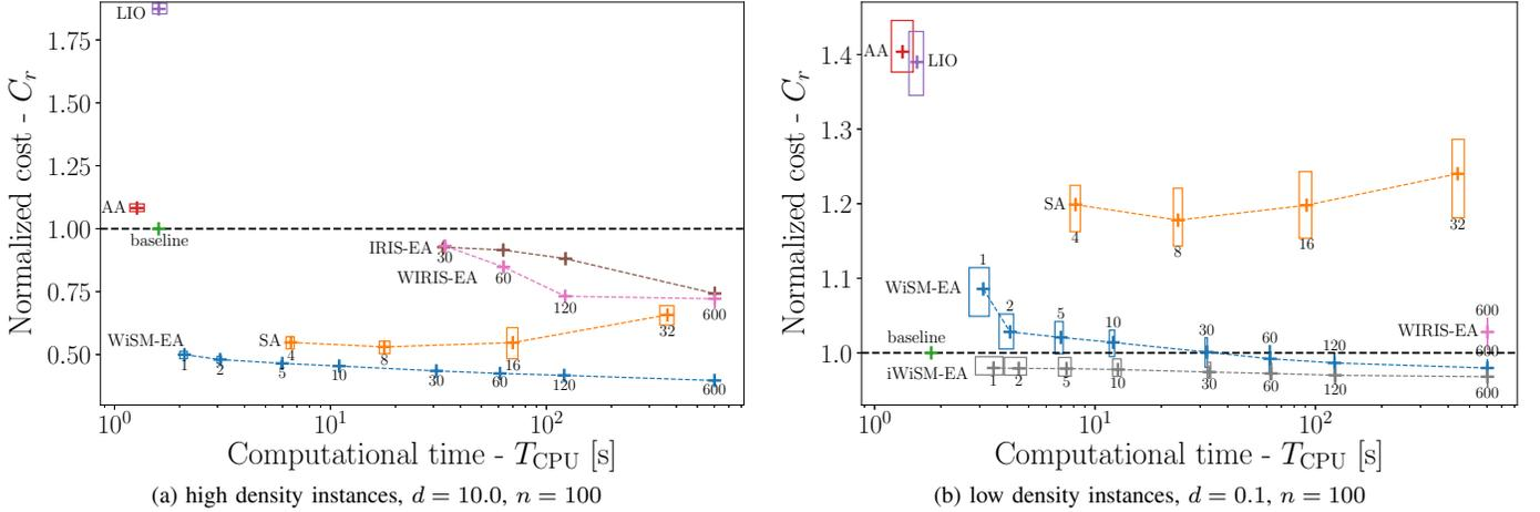
Fig. 4. Performance of the evaluated DTSP solvers in high ( $d = 10$ ) and low ( $d = 0.1$ ) density instances with  $n = 100$  target locations. The achieved normalized cost  $C_r$  is shown according to the required computational time or a given time limit (for the WiSM-EA). For  $d = 0.1$ , the iWiSM-EA refers to the proposed WiSM-EA with the initialization of the population by the solution of the Euclidean TSP provided by the Concorde solver.
