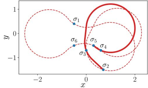
Fig. 2. A solution of the closed DTP with  $n = 6$  locations with a corresponding instance of the Open DTP over four locations  $\Sigma_{3,2}$  (thick solid line).
