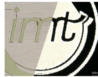
Fig. 23: Micrograph of successful areal ablation. Left side shows the sample directly after laser irradiation. Right hand side picture was taken after ultrasonic cleaning with through light illumination only. Coating dust is completely removed.
