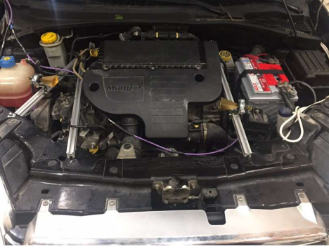
Fig. 2. Transmitter and receiver antennas in the engine compartment.
