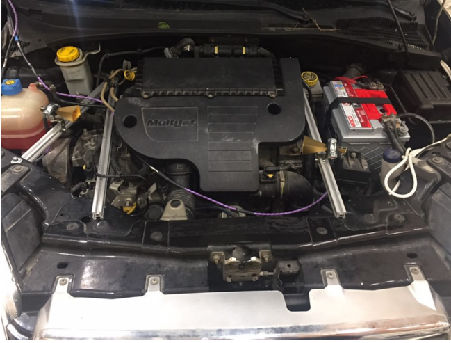
Figure 2: Transmitter and receiver antennas in the engine compartment
