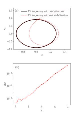
FIG. 4. (a) Projection of the TS trajectory, determined by the centroid search. Trajectories are plotted over 2.5 periods for both, the trajectory determination with and without the stabilization on the NHIM. (b) Distance  $\Delta x$  between the x-coordinates of the two trajectories calculated with and without the stabilization over two periods. Within one period the separation is two orders of magnitudes smaller than the actual motion in x direction.
