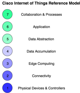
Figure 1. 7-layer IoT architecture proposed by Cisco
