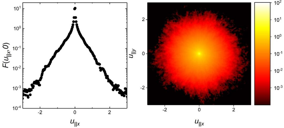
Figure 4. Probability density function for the velocity parallel to the polarization. Left Panel: histogram of  $F(u_{\parallel x}, 0)$ . Right Panel: heat map of the probability density function  $F(u_{\parallel x}, u_{\parallel y})$  in the  $(u_{\parallel x}, u_{\parallel y})$  plane. In both panels,  $u_{\parallel}$  is  $v_{\parallel}$  rescaled in natural units of velocity.
