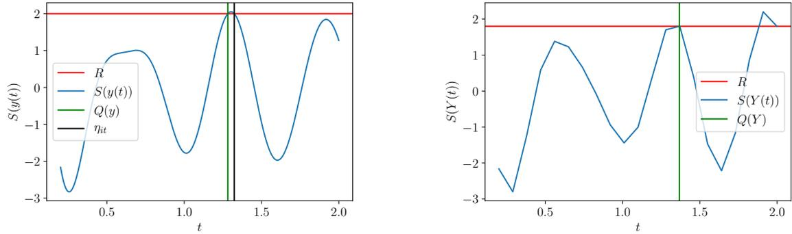
(a) Figure detailing issue with iterative methods in §4.4.1 and §4.4.2 when the numerical solution is not accurate near the event. The iterative methods result in  $t^* = \eta_{it}$ , which is the second occurrence of the event rather than the first. This figure specifically details the case when  $R = 2$ .
