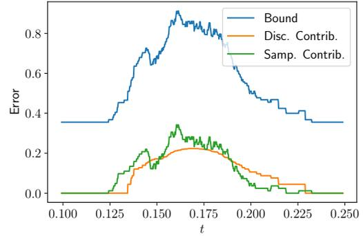
(b) Breaking the error bound into sampling and discretization contributions for the problem in §5.1 when using 100 samples. The sampling and discretization contributions are computed as the first and second terms of (43), respectively.
