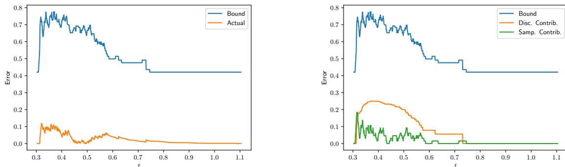
(a) Comparing error bound (43) to true error for example in §5.2 when using 1000 samples for the nominal CDF and 80 samples for the numerical CDF.
