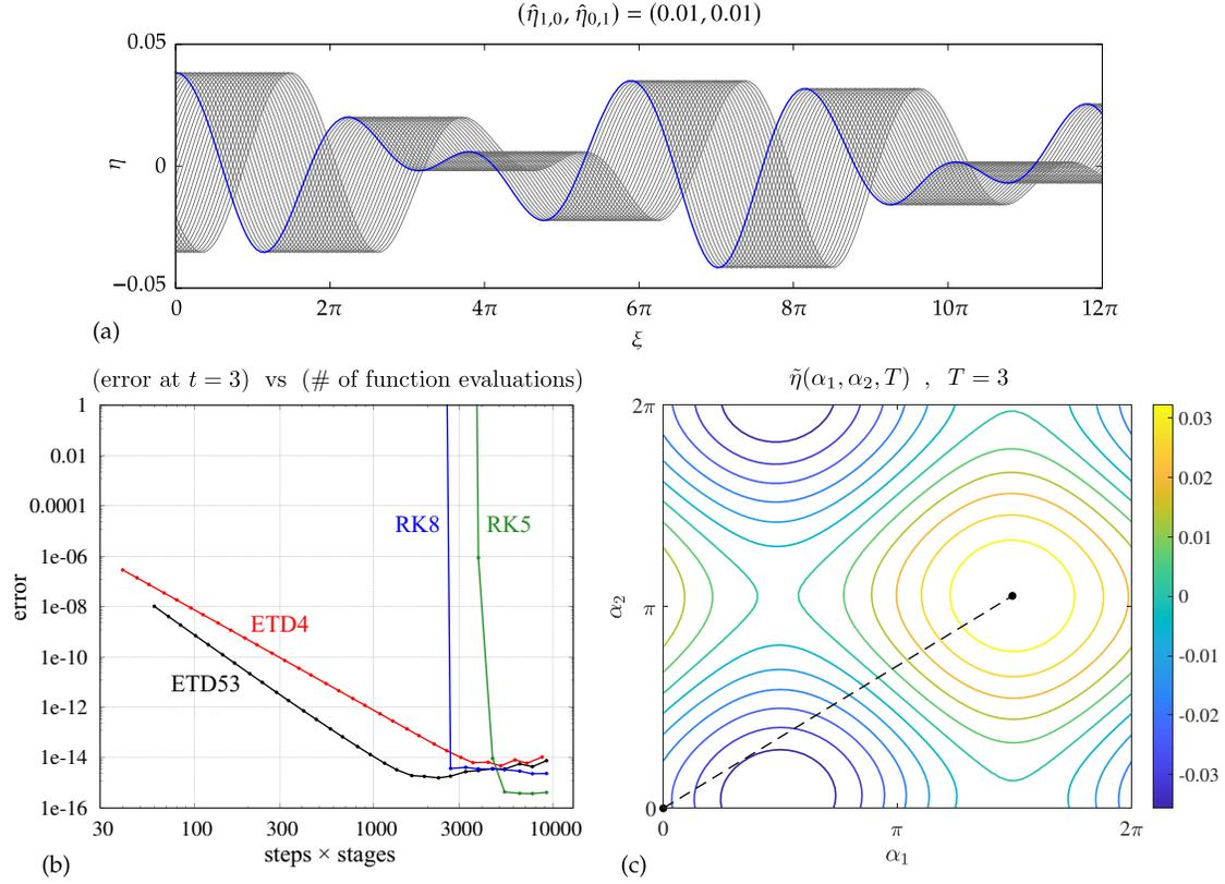
FIGURE 1. Time evolution of a quasi-periodic traveling water wave computed in [76] and a convergence plot comparing the accuracy and efficiency of the proposed time-stepping schemes.
