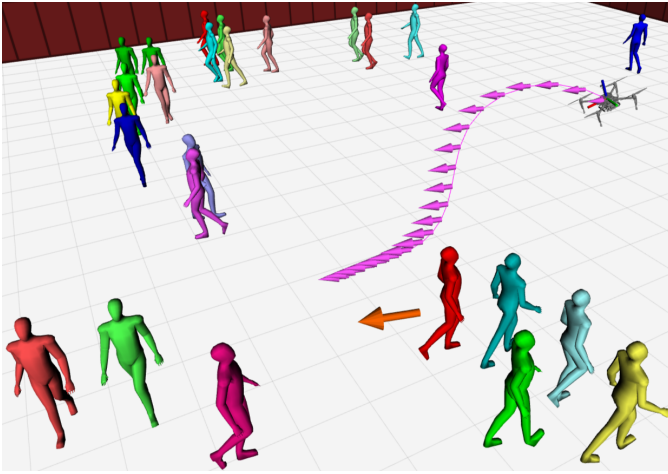
Figure 4: Crowd collision avoidance simulation with 30 pedestrians. The orange arrow represents the moving reference position. The robot pose and predicted trajectory are indicated by the frame and the purple arrows respectively.
