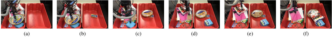
Fig. 11: Random picking. The robot is requested to pick and place of all objects located in left bin (source) to the right bin (destination).
