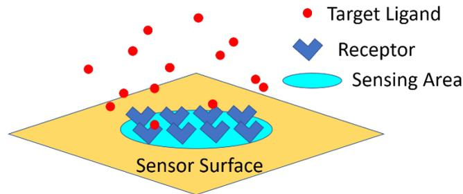
Figure 4, Schematic representation of a molecular sensing device. Receptors immobilized in a sensing area bind target ligands in a sample.
