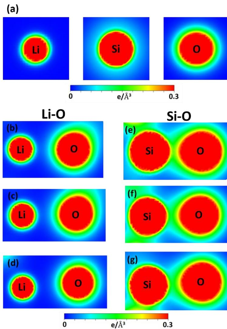
**Figure 5** The spatial charge density distribution for (a) the isolated (Li, Si, O) atoms. The shortest/medium/longest (b)/(c)/(d) Li-O and (e)/(f)/(g) Si-O bonds
