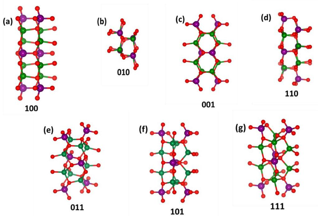
**Figure S1(a)-S1(g)** Projections of  $\text{Li}_2\text{SiO}_3$  onto distinct planes: (a) (100), (b) (010), (c) (001), (d) (110) (e) (011), (f) (101), (g) (111) where the Li, Si and O atoms correspond to the green, purple and red balls, respectively.
