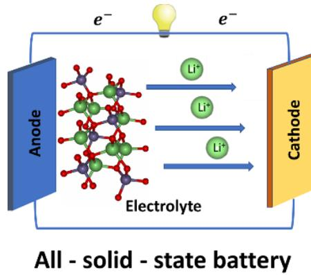
**Figure 1** All -solid-state  $\text{Li}^+$  based battery with the electrolyte of three dimension ternary  $\text{Li}_2\text{SiO}_3$
