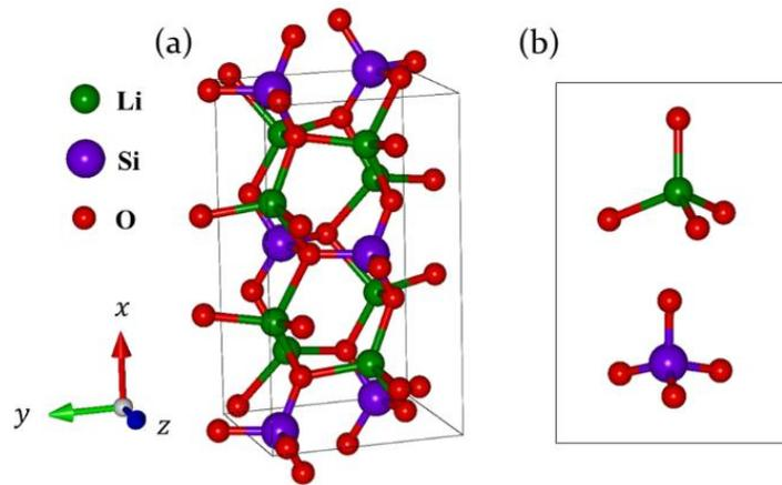
**Figure 2** (a)The optimal lattice structure of  $\text{Li}_2\text{SiO}_3$  under the orthorhombic symmetry with 24 atoms in a unit cell of lattice constants  $a = 5.440 \text{ \AA}$ ,  $b = 9.467 \text{ \AA}$  and  $c = 4.719 \text{ \AA}$  (b) Two kinds of chemical bondings: Li-O and Si-O.
