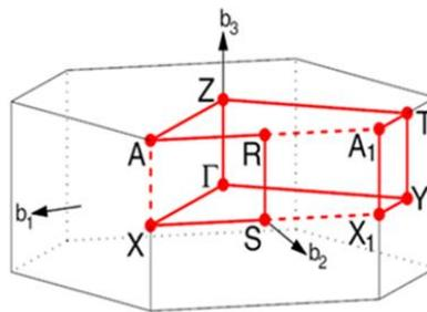
**Figure 3** The first Brillouin zone with the high-symmetry points within the three orthogonal axes.
