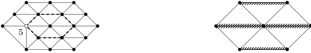
FIGURE 10. Left: Exemplary triangulation (\mathcal{T}, \text{ref}_{\mathcal{T}}) . The vertex v with \#\tilde{\mathcal{R}}_v = 5 (in white) blocks all vertices along the loop (dotted) from deletion. These vertices are connected through red middle elements. Right: Initial triangulation (\mathcal{T}_0, \text{ref}_{\mathcal{T}_0}) of the left mesh.
