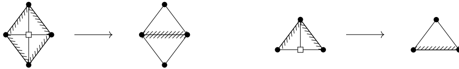
FIGURE 16. Compatible patches as shown in [7]. The nodes v (white squares) have the property v \in \mathcal{N}_{\text{new}} and \#\mathcal{R}_v \in \{2, 4\} and can thus be eliminated in a coarsening step. Reference edges are shown as hatched lines.
