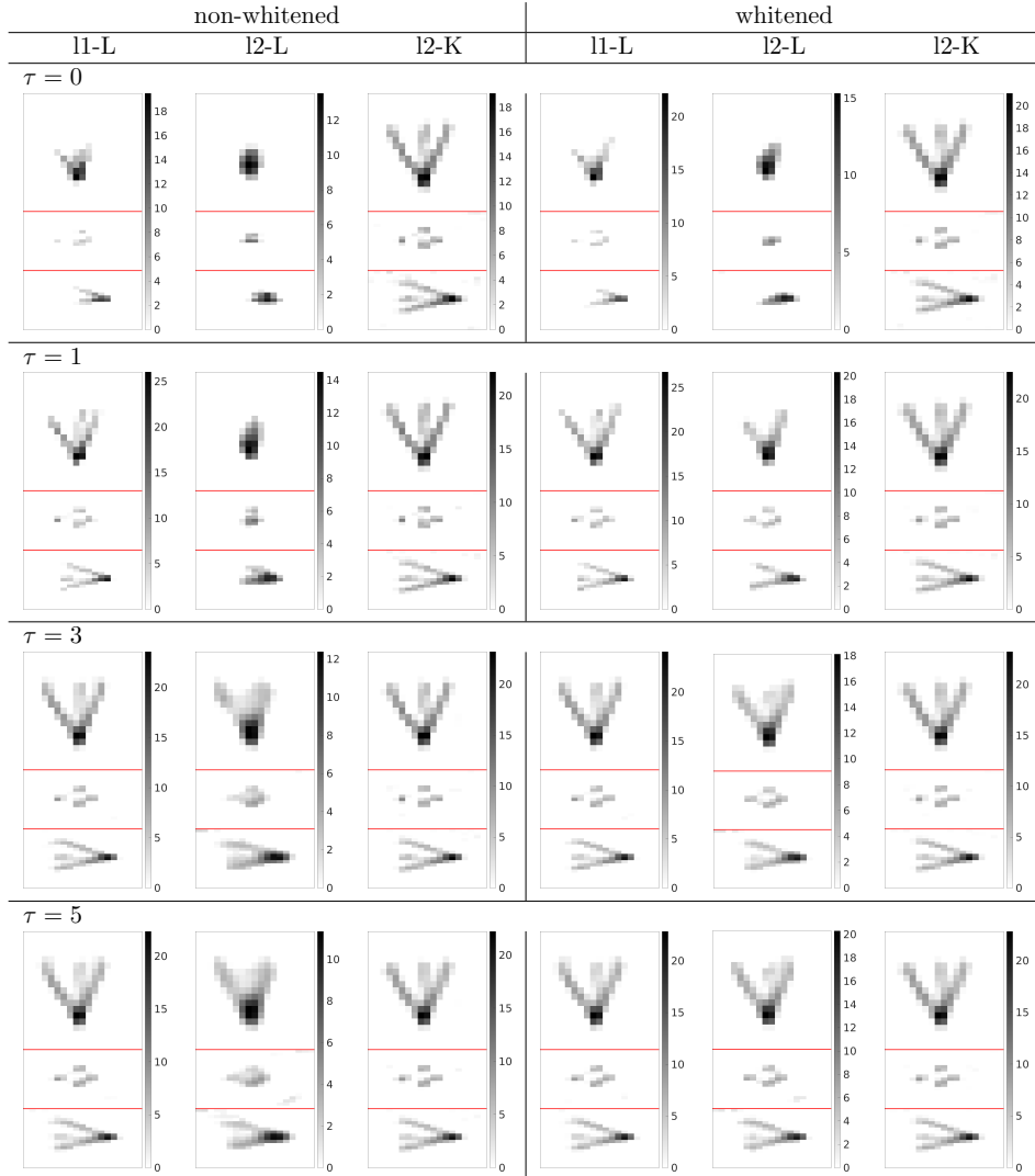
Figure 18: Fig. 9 with inverted colormap: “Resolution” phantom reconstructions, SSIM-optimized \alpha and iteration number N (for l2-K only) according to Table 2.
