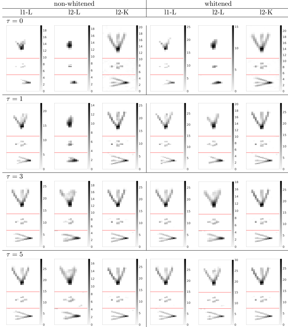
Figure 16: Fig. 7 with inverted colormap: “Resolution” phantom reconstructions, PSNR-optimized \alpha and iteration number N (for l2-K only) according to Table 1.
