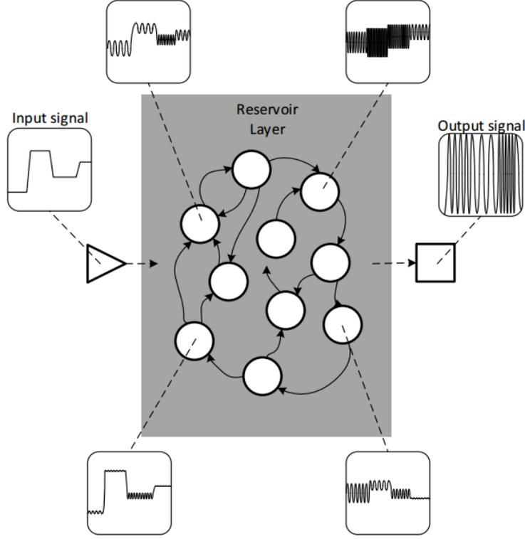
Fig 2. Versatility of states of dynamical reservoir presented on the example of the frequency generation. Adapted from [18].
