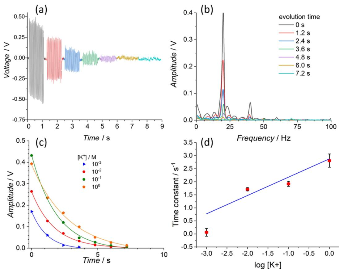
Fig 8. Exemplary response of the studied reservoir computing sensing system with feedback loop at high  $K^+$  ion concentration (a). Fourier transform spectra of each and every repeated signal package as a function of evolution time (b). Signal amplitudes of the first component (20 Hz) as a function of evolution time and potassium ion concentration (c), which enabled calibration of the time constants as a function of potassium concentration (d).
