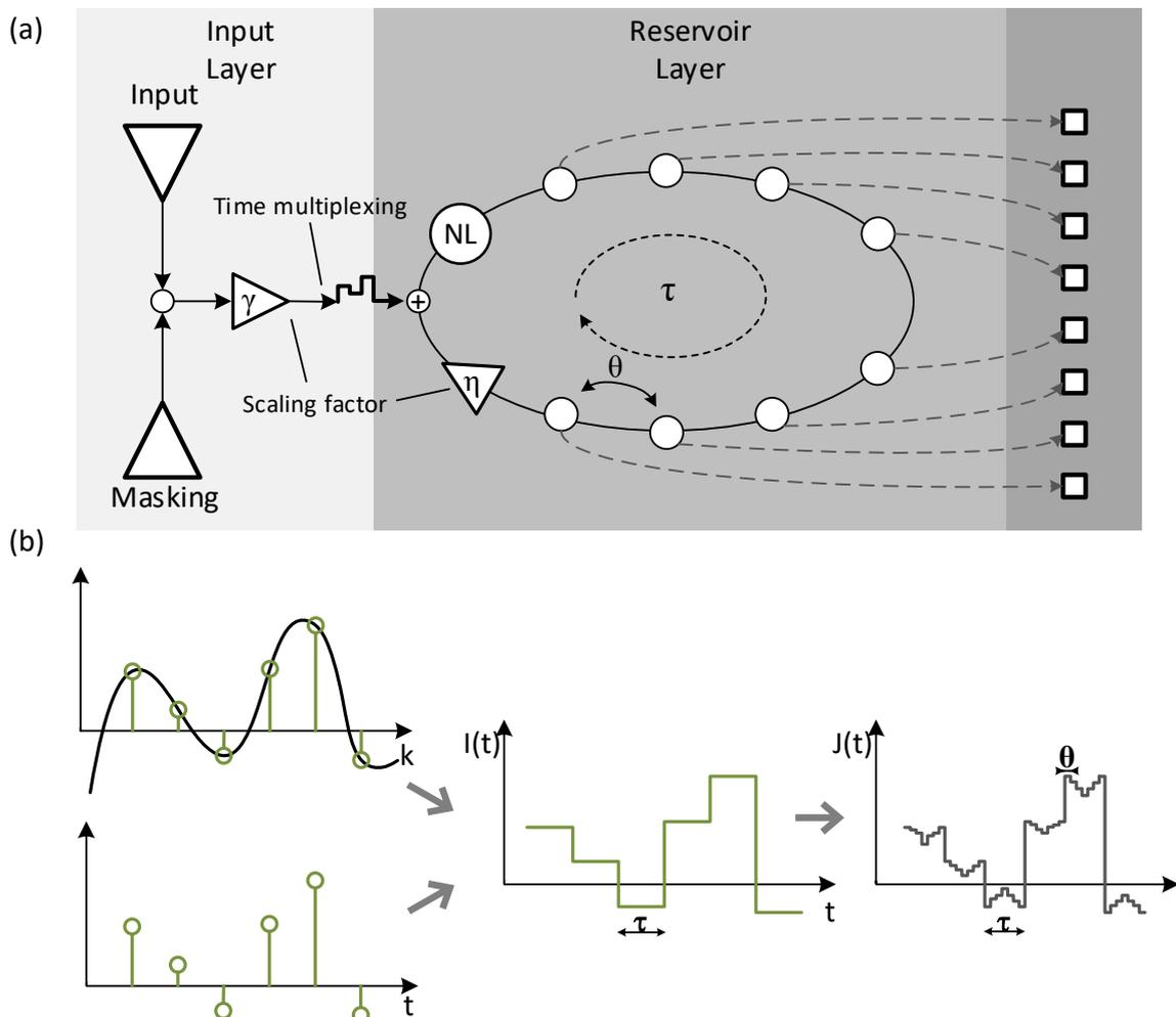
Fig 3. A schematic structure of the delay-based reservoir computing device.  $\tau$  is the length of the delay line,  $\theta$  is the distance between neighbouring nodes. Masked input is scaled by scaling factor  $\gamma$ , as well as signal in the delay line, which is scaled by feedback strength  $\eta$ . Scaling operations are often required to ensure that the signals in the reservoir are not saturated nor suppressed. Determination of scaling factors is optimised through numerical methods or
