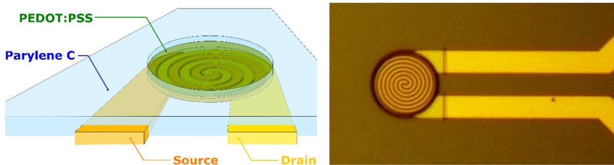
Fig. 6. Design (left) and optical microscopy image (right) of PEDOT:PSS organic electrochemical transistor.
