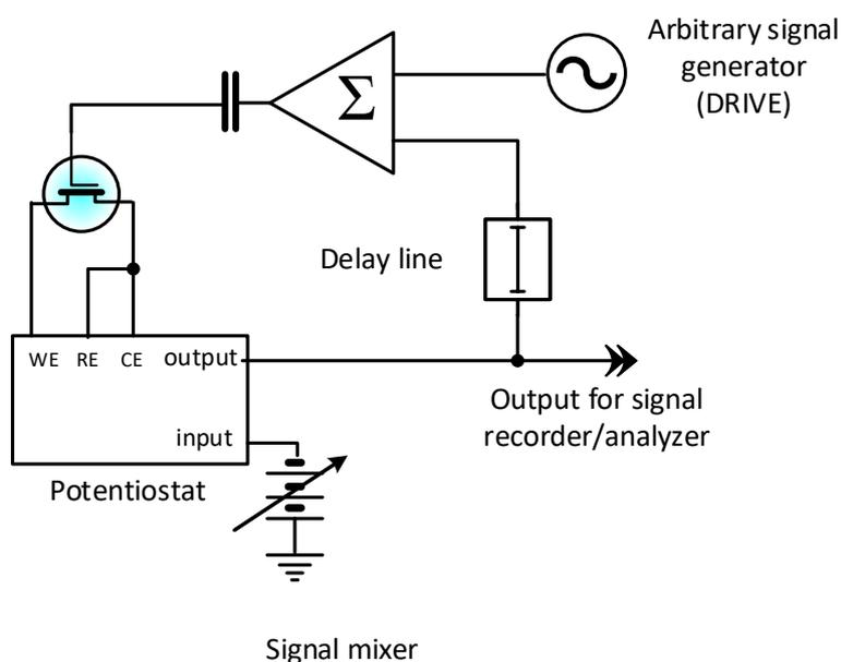
Fig. 7. Connection diagram of a reservoir sensing system with OECT as an active element. Potentiostat input controls the potential source, the output is the analog current monitor.
