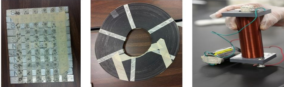
Fig 1. The magnetic field arrangements for the experiment. (a) static field arrangement, (b) Random field generating coil and (c) Electromagnetic field inside the coil which perfectly fits a test tube attached with 3V battery.
