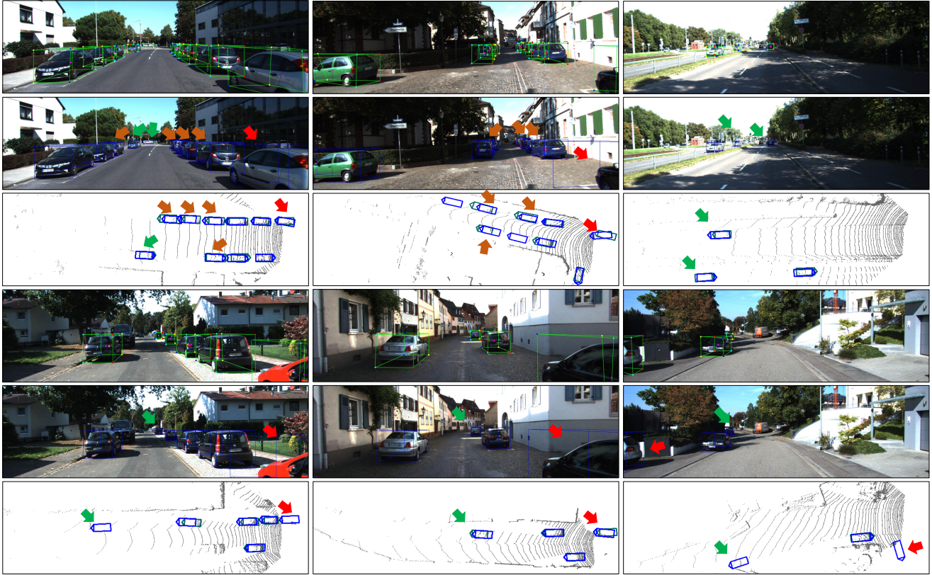
Figure 4. Qualitative results of our 3D detection. From top to bottom are keypoints, projections of the 3D bounding box and bird’s eye view image, ground truths in green and our results in blue. The crimson arrows, green arrows, and red arrows point to occluded, distant, and truncated objects, respectively.
