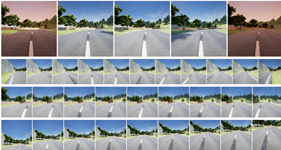
Fig. 5: Example images at the same point showing, from top to bottom, the effect of times of day, lateral offset, camera yaw angle and camera pitch angle.
