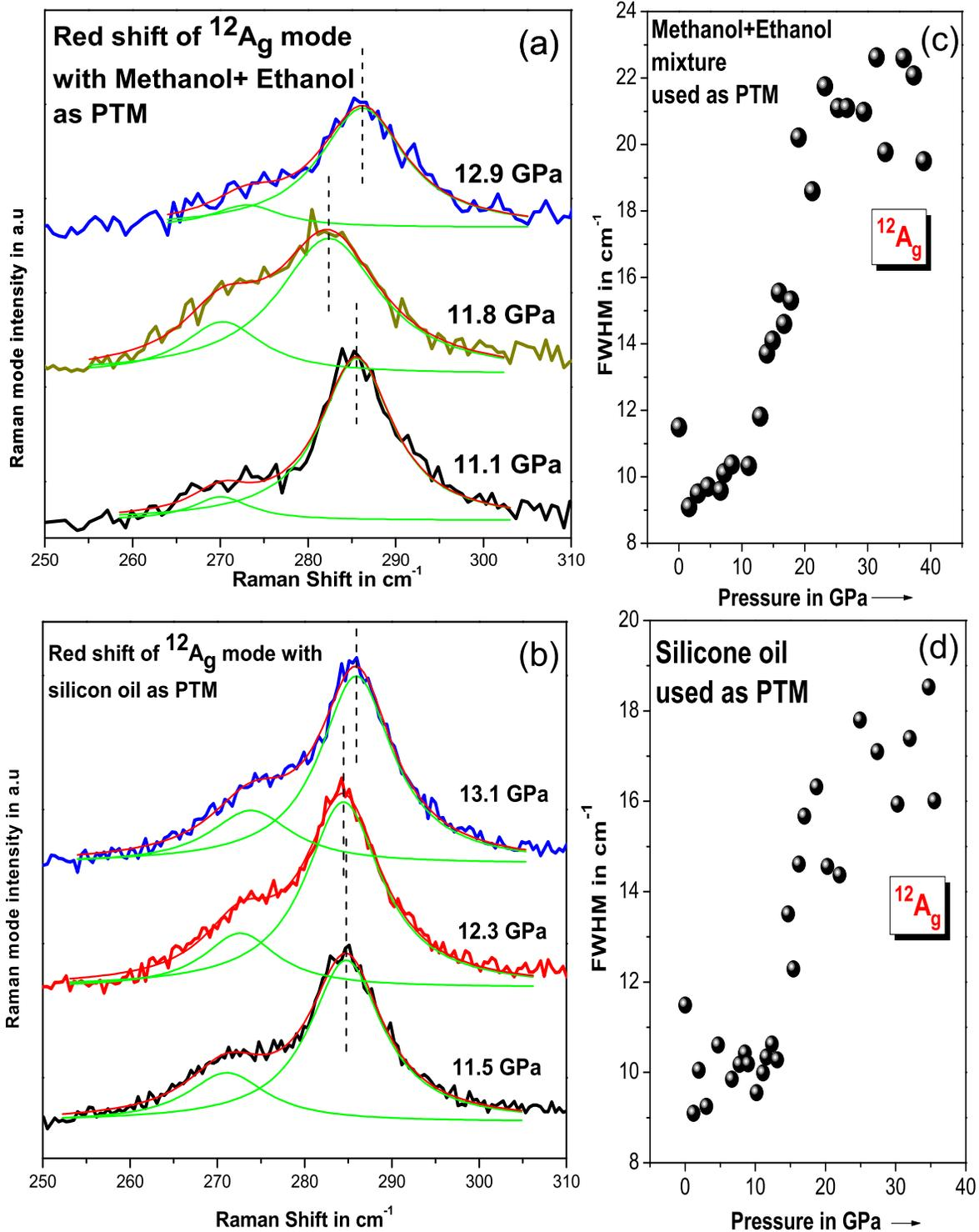
Figure 6. Redshift of  $^{12}A_g$  mode using (a) Methanol-Ethanol mixture as PTM, (b) Silicone oil as PTM. Pressure variation of FWHM for  $^{12}A_g$  mode using (c)Methanol-Ethanol mixture as PTM, (d) Silicone oil as PTM.
