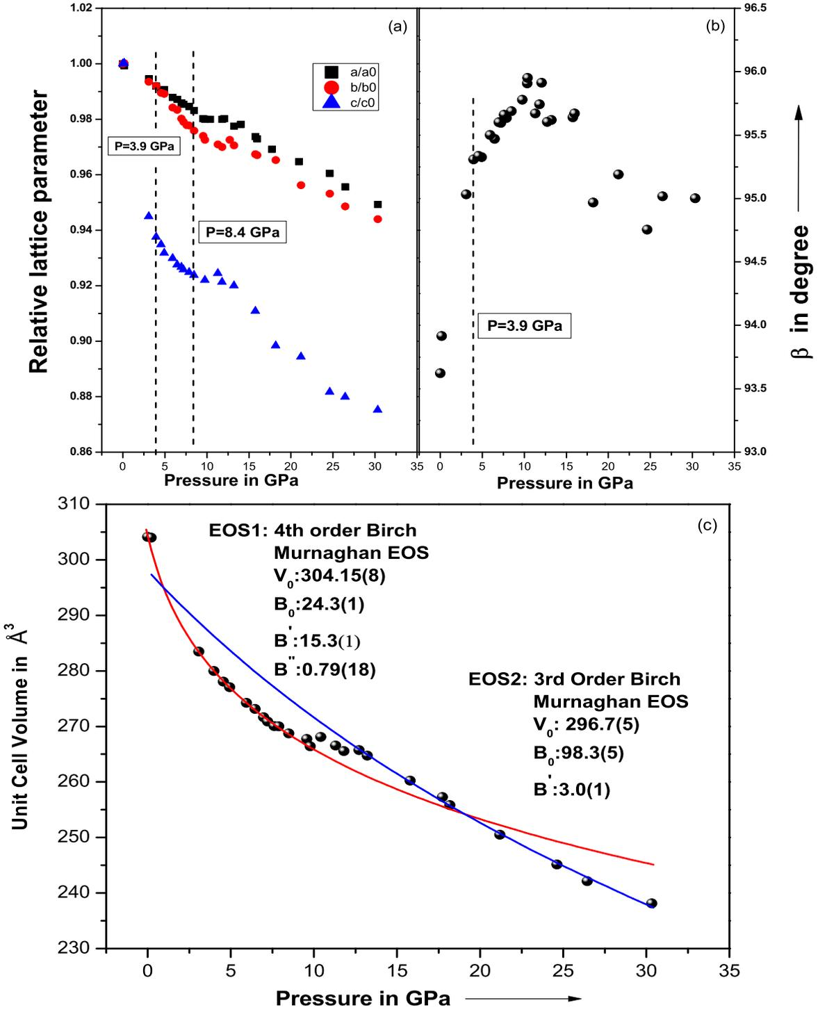
Figure 2. (a) variation of  $a/a_0, b/b_0$  and  $c/c_0$  with pressure. The dashed vertical lines indicate pressure points showing the anomalous changes in lattice parameters. (b) Variation of lattice angle  $\beta$  with pressure. (c) The variation of unit cell volume with applied pressure. The lines through data points show the EOS fits.
