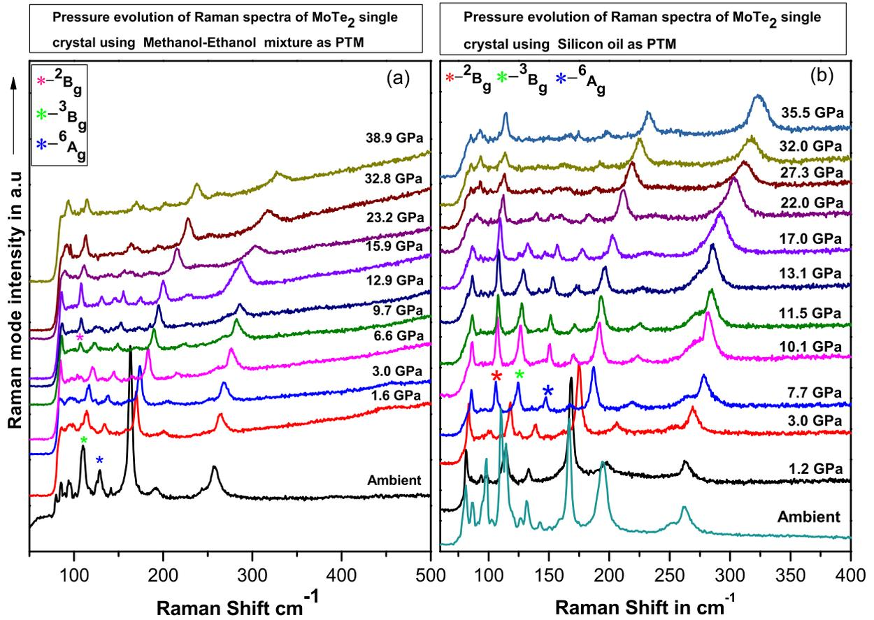
Figure 4. (a) Pressure evolution of Raman Spectra using Methanol-Ethanol mixture as PTM and 532nm laser as excitation source. (b) Pressure evolution of Raman Spectra using Silicone oil as PTM and 488nm laser as excitation source.
