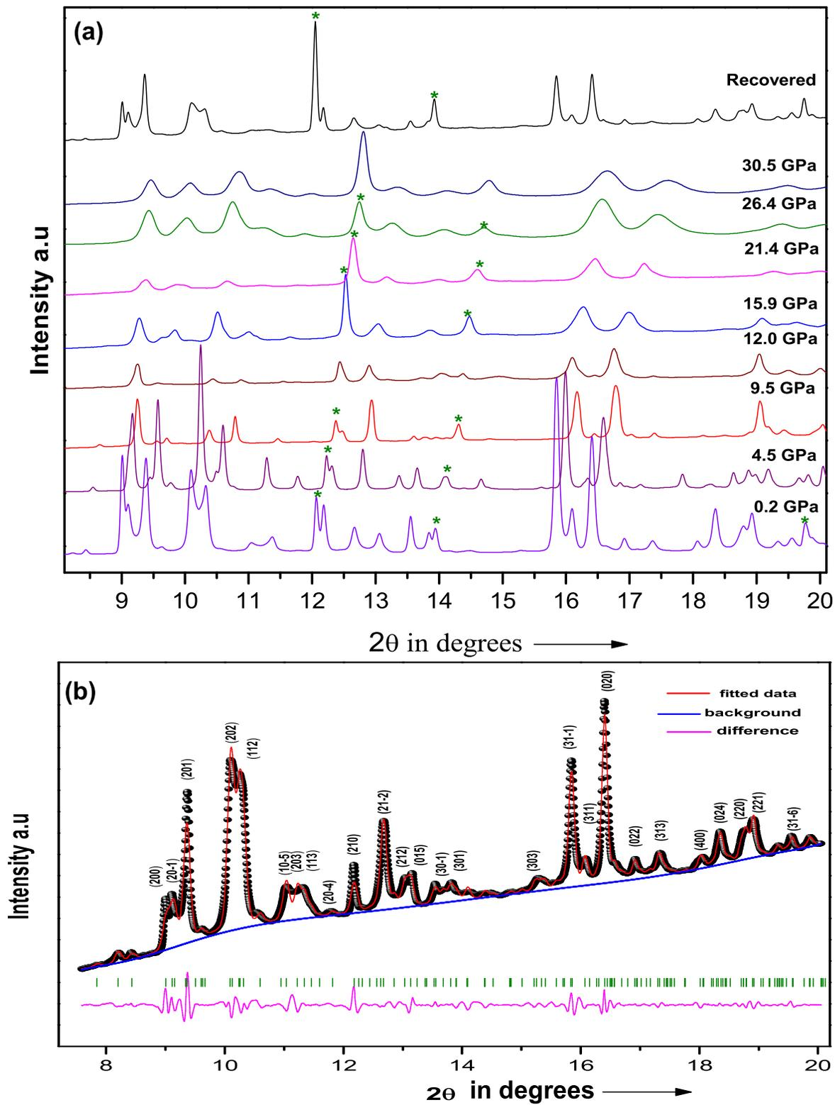
Figure 1. (a) pressure evolution of XRD patterns at selected pressure points and (b) Leblat profile fitting of XRD pattern at ambient pressure.
