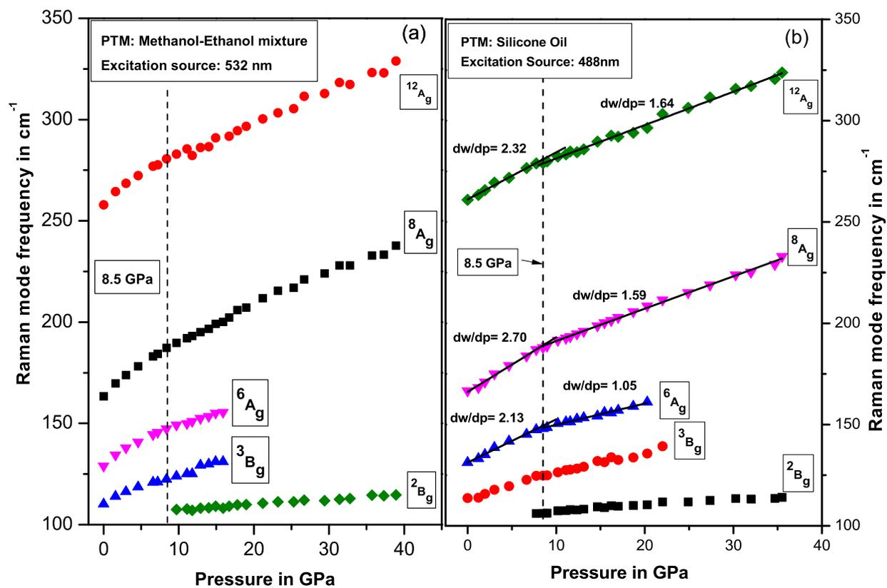
Figure 5. Variation of few selected Raman mode frequencies with pressure, using (a) Methanol-Ethanol mixture as PTM and (b) Silicone oil as PTM. Around 8.5 GPa a change in slope is observed for most of the modes.
