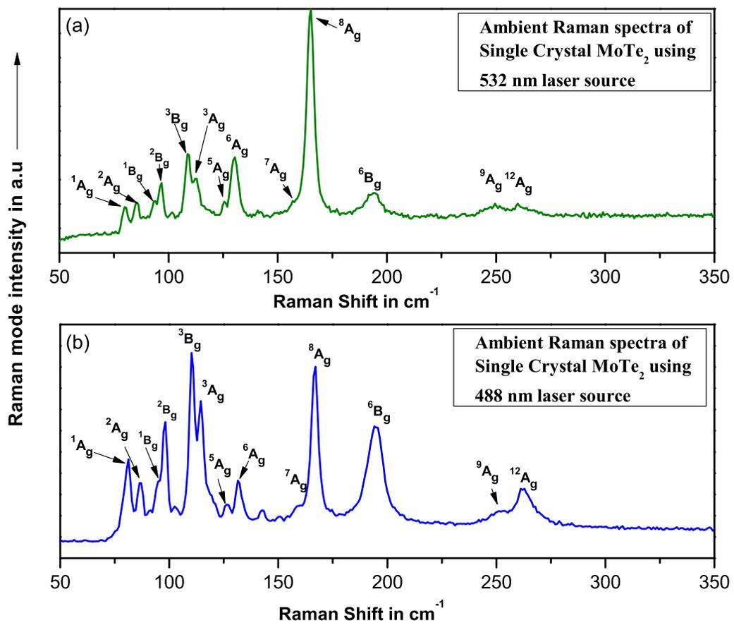
Figure 3. (Colour online) Ambient Raman Spectra using 532nm and 488nm excitation source. All the modes detected are shown in figure.
