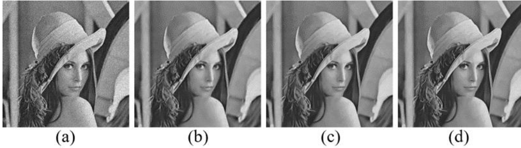
Figure 4 The denoising effects of different methods. (a) is the noised image; (b)-(d) are the denoising results of BLS-GSM method, BM3D method and MLFE-BM3D method, respectively.
