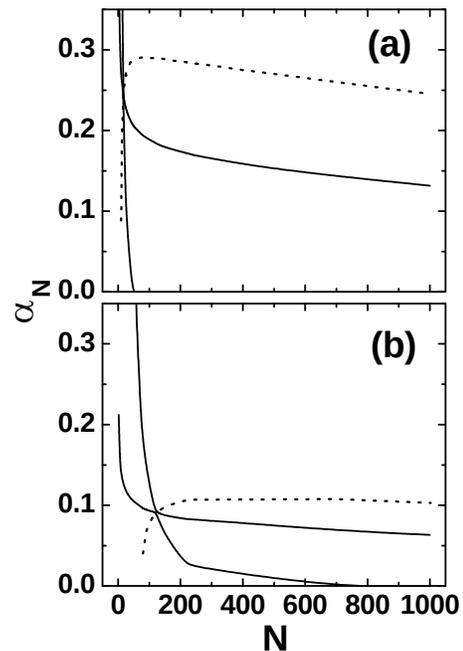
FIG. 17. Points in the plane  $(\alpha_N, \gamma)$ ,  $\alpha_N = \alpha/\sqrt{N}$ , at which steady Schrödinger-cat states occur, are displayed in dashed-line. The solid-line corresponds to the contour plot of Exceptional Points. We have considered the case  $d_- = 0$ , with  $D = 2.88$  [GHz] and  $E = 0.026$  [GHz]. In panel (a) and (b) we plot results for  $g = 0.02$  [GeV] ( $\gamma_N = 1/(13\sqrt{N})$ ) and  $g = 0.052$  [GeV] ( $\gamma_N = 2/\sqrt{N}$ ), respectively.
