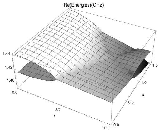
FIG. 2. Behaviour of the real components of the eigenvalues  $E_{1-}$  and  $E_{2-}$  as a function of the parameters  $\gamma$  and  $\alpha$ , for  $\Delta = 2D$ , and  $E = 0.026$  [GHz].
