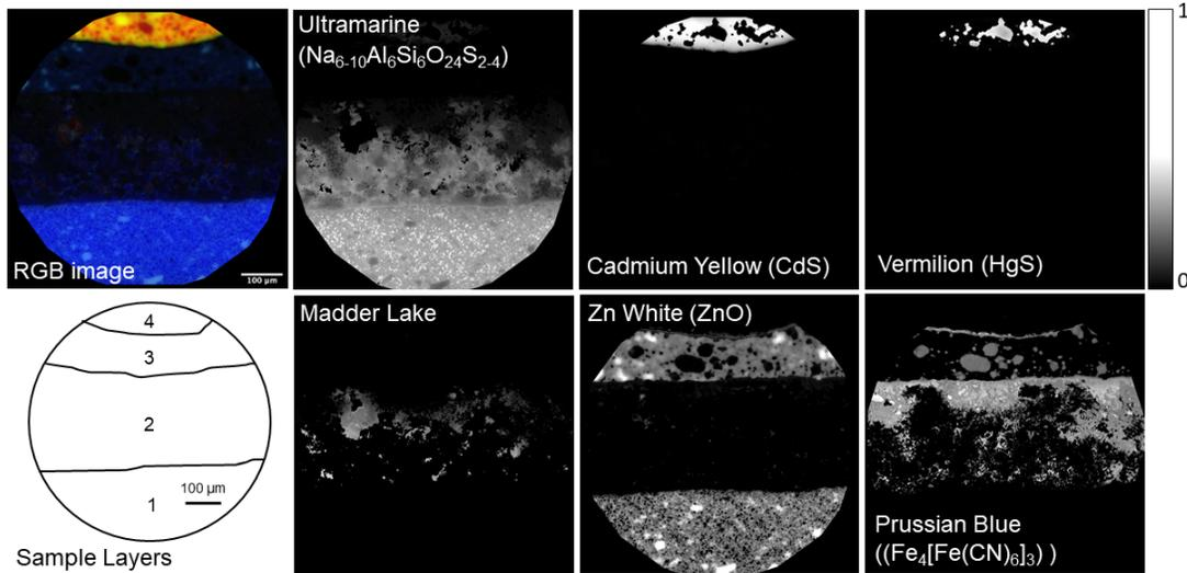
**Figure 4.** Cross-section of the multi-layered mockup sample including the reconstructed RGB image and the corresponding pigment maps created by sparse modeling of the diffuse spectral dataset. The maps were created using an orthogonal matching pursuit (OMP) algorithm with a dictionary comprised of pure pigment spectra (ultramarine, cadmium yellow, vermilion, madder lake, zinc white, and Prussian blue). Distribution weights are normalized between 0 and 1 on a per pixel basis.
