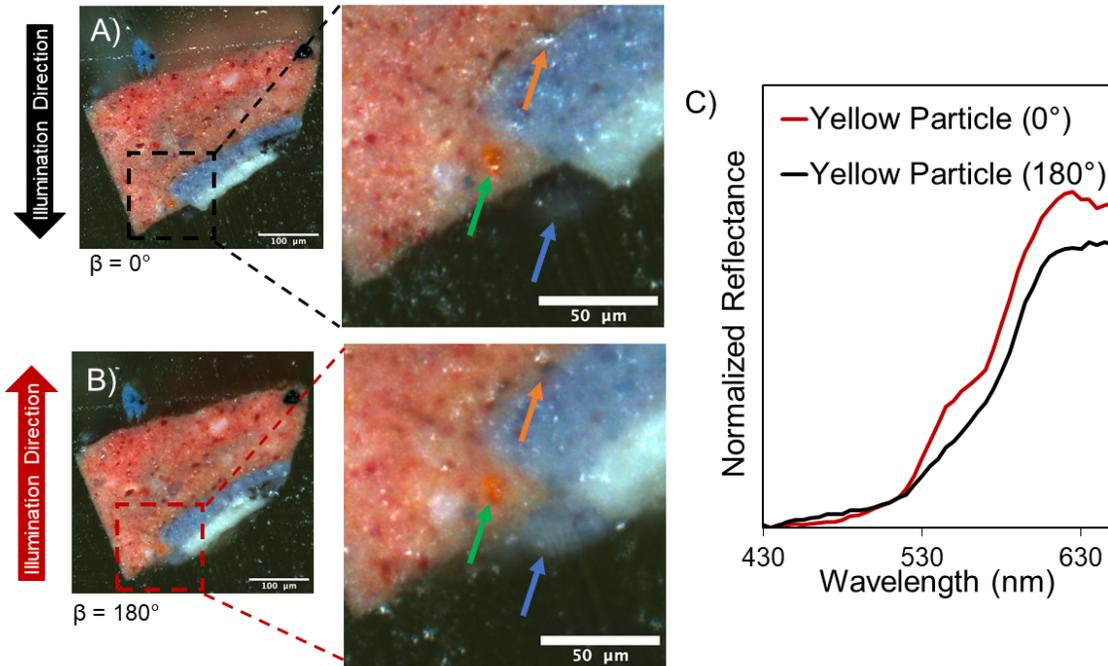
**Figure 2.** RGB images of a cross section from Picasso's *La Miséreuse accroupie* acquired at A)  $\beta = 0^\circ$  and B)  $\beta = 180^\circ$ . The arrows highlight distinct differences between images due to illumination direction. C) Reflectance spectra extracted from the yellow-orange particle at  $\beta = 0^\circ$  (red trace) and  $\beta = 180^\circ$  (black trace). See Movie S1 for multiple illumination angles.
