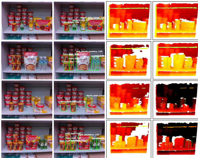
Fig. 5: Qualitative results of the perception algorithm captured in a real convenience store. Each row captures a different scenario. The four columns depict from left to right the input image, 2D detection results, input point cloud and box fitting result. Bounding boxes are depicted in green for 2D and 3D case.
