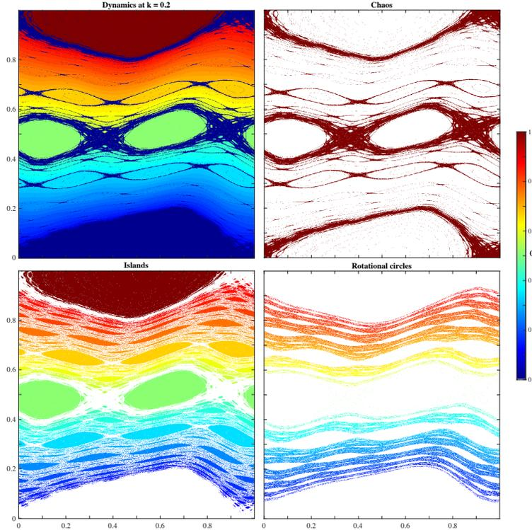
Figure 21: The dynamics of the asymmetric two harmonic map (26) for  $k = 0.2$  and  $\psi = 0.7776$ . The weighted Birkhoff method distinguishes chaotic orbits (upper right), islands (lower left), and rotational circles (lower right). The rotation number of each nonchaotic orbit is color-coded (color bar at right). The computations were performed for a grid of  $1000^2$  initial conditions in  $[0, 1]^2$  with  $T = 10^4$  with distinguishing criteria in (23).
