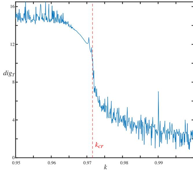
Figure 15: Computation of  $dig_T$  for the golden mean circle for  $T = 2(10)^4$  for 500 values of  $k \in [0.95, 1.00]$ . Continuation is used to find the initial condition  $(0.321, y_0)$  that has  $\omega = \gamma^{-1}$ . The drop of  $dig_T$  from 12 to 6 indicates that the circle is destroyed for a parameter value in  $(0.9706, 0.9731)$ .
