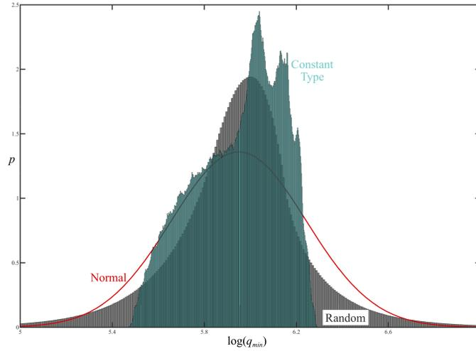
Figure 10: Probability density of  $\log_{10}(q_{min})$  computed by appendix Algorithm 2 with  $\delta = 10^{-12}$  for  $10^8$  randomly chosen numbers in  $(0, 1)$  (black). This distribution has mean 5.9497, mode 5.9662, standard deviation  $\sigma = 0.29333$ , and kurtosis 6.3073. The red curve shows the normal distribution with the same mean and standard deviation. Also shown is the histogram for  $10^8$  randomly chosen numbers of constant type with  $A = 10$  (green).
