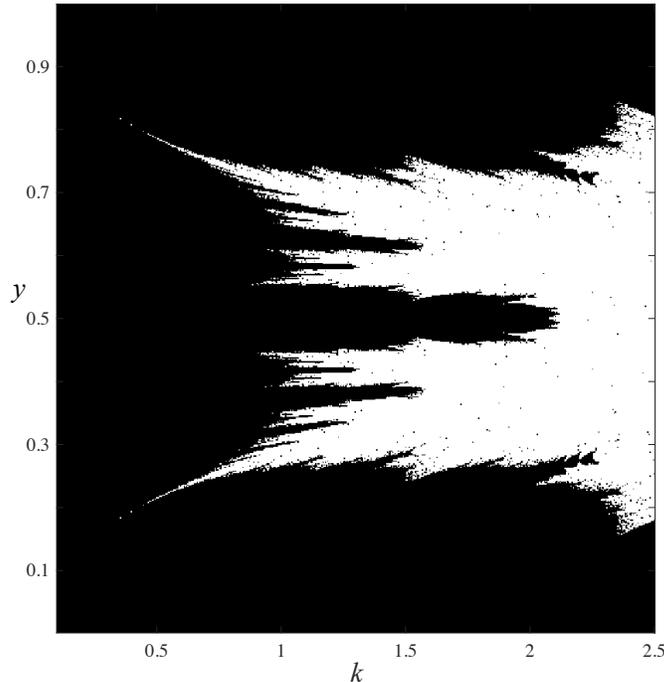
Figure 7: Chaotic region of the standard map with  $x_0 = 0$  for  $y \in [0, 1]$  and  $k \in [0.1, 2.5]$  using a time series  $\{\sin(2\pi x_t) : 0 < t \leq 1000\}$  and the 0–1 method of [GM09]. An orbit is deemed to be chaotic (colored white) if the 0–1 parameter  $K_{median} > 0.5$ .
