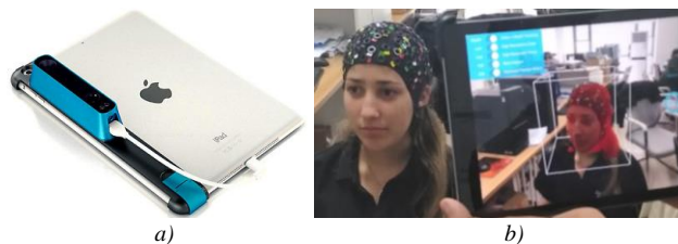
Fig.2: a) Occipital structured sensor ST01 [10] and iPad A1893 [13]. b) Scanning process around the subject.
