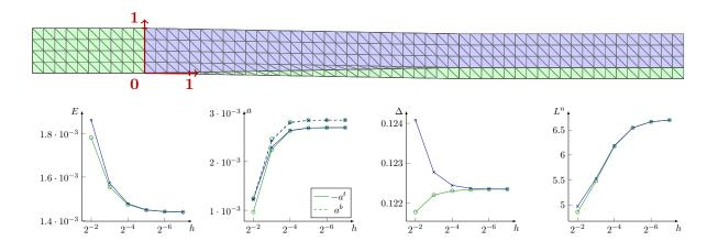
Figure 6 – Top: Coarsest finite element mesh,  $h = 2^{-2}$ ,  $\square$  type. Bottom: Convergence plots for the total energy and the four optimization parameters (the two curvatures  $-a^t$  and  $a^b$ in the second plot). In each plot the results for  $\square$  (blue x markers, corresponding to the mesh depicted on top) and  $\square$  (green circle markers) grids are shown for successive refinement by quadrisection. A symmetric needle would have  $\Delta = 0.125$ .
