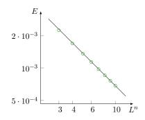
Figure 4 – Linearized elastic energy of the optimal needle shape for different values of  $L^n$ , demonstrating that there is no fixed length scale in the linearized case. The black line shows the slope of  $1/L^n$ .
