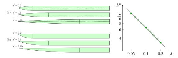
Figure 3 – Optimal needle shape for different values of  $\delta$  in the (a) reference and (b) deformed configuration, scaled for clarity by a factor of 4 vertically as in Figure 2 (b) and (c). The right panel shows the needle length  $L^n$  as a function of  $\delta$  (the filled circles mark the configurations on the left). The black line shows the slope of  $1/\delta$ .
