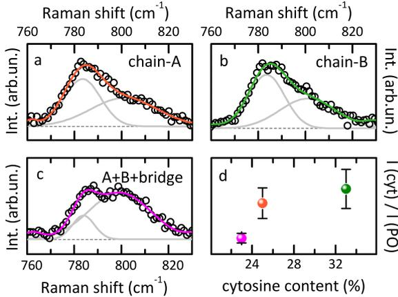
Figure 6: Gaussian deconvolution of the SERS spectra of chain-A (a), chain-B (b) and bridge hybridized sample (c) in the  $760\text{--}830\text{ cm}^{-1}$  spectral region, where the band assigned to the cytosine and O-P-O vibrations is visible. In panel d, the ratio between the intensity of the low to high frequency components of the band is correlated with the concentration of cytosine in the probed sequences.
